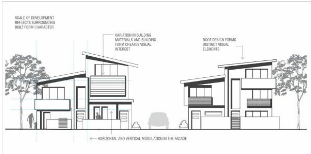
Figure 6.7 Building design elements
