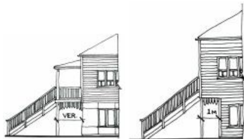
Figure 6.74 - Appropriate enclosures to the ground floor
